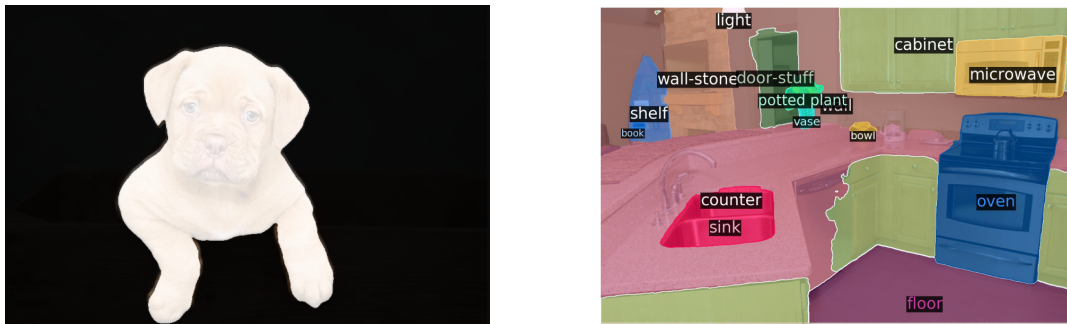
Figure 1.2: Segmentation. In the left image, a model recognizes (segments) the pixels corresponding to a dog. All other pixels are classified as "not dog". In the right image, a multiclass segmentation model identifies the different objects in a kitchen (source: Carion et al. (2020)).
