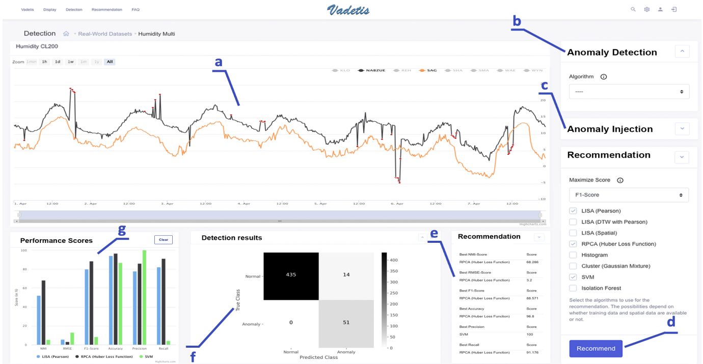
Fig. 2: VADETIS allows to (a) visualize (raw and normalized) time series with their metadata and to (b) perform anomaly detection on them. Users can (c) generate anomalies in specific time series while specifying their type, scale and frequency. They can also (d) choose a performance metric and the tool then evaluates a set of detection techniques, compares their performance, and recommends the optimal technique. The tool provides a GUI that enables displaying time series with anomalies highlighted, as well as the results of the detection/recommendation (e, f, and g).
